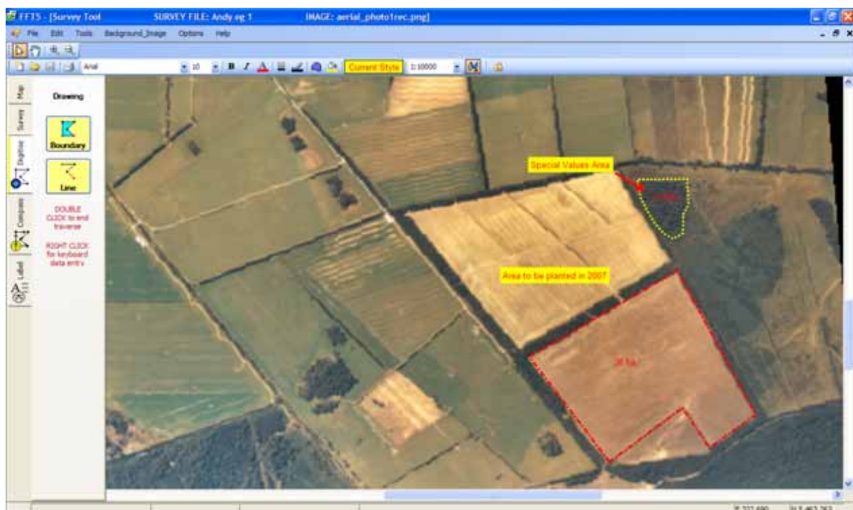
Figure 2 The Survey tool can be used to calculate and annotate areas using an aerial photograph or satellite image in the background
